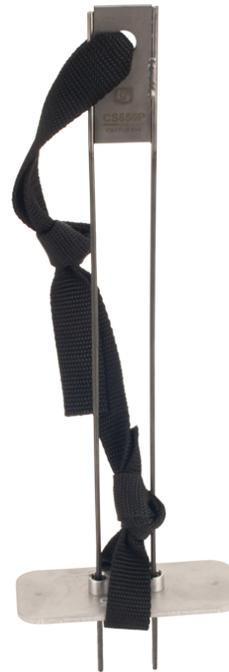
The CS650G makes inserting CS616 easier in dense or rocky soils. This tool can be hammered into the soil with force that might damage the sensor if the CS650G were not used. It makes pilot holes into which the rods of the sensors can then be inserted.
