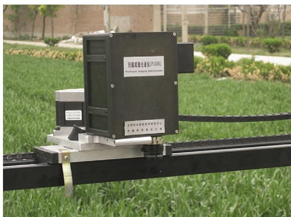
Fig. 1 – Pushbroom imaging spectrometer.
