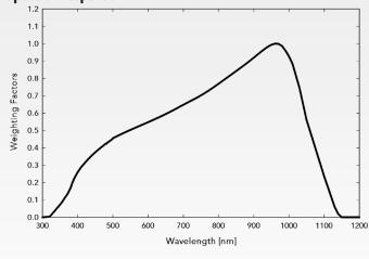
Spectral response estimate of Apogee siliconcell pyranometers. Spectral response was estimated by multiplying the spectral response of the photodiode, diffuser, and adhesive. Spectral response measurements of diffuser and adhesive were made with a spectrometer. and spectral response data for the photodiode were obtained from the manufacturer.
