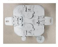
The attached screw holders are used to secure the device. The holders should be inserted into slots located on the back side of the instrument. The Auxanometer should be installed at the base of the tree trunk under study. A cord exceeding the height of the tree must be attached to the ring of the device. The free end of the cord shall be fixed in tension at a top of the tree in any convenient way. With further growth of the top of the tree, the cord will be pulled out of the device.
