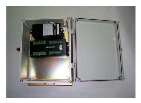
The HL20 datalogger is a powerful data acquisition system suitable for various applications including meteorology, hydrology, ambient air pollution, agriculture, industry, wind and solar power energy, water quality & resource, ground water, soil erosion research, debris flow, geotechnical measurement, etc. It can work as a stand-alone station or be operated and controlled by remote IBM compatible PC or through dedicated Ine, dial-up modem or GSM modem or Internet as a monitoring systems network.
