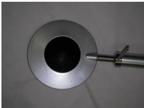
ENR Net Radiometer measures the net radiation across a surface, from near ultraviolet (UV) to far infrared. ENR Net Radiometer is designed and constructed to used in any weather conditions for routine measurement of net radiation, which is the balance between incoming and outgoing radiation.
