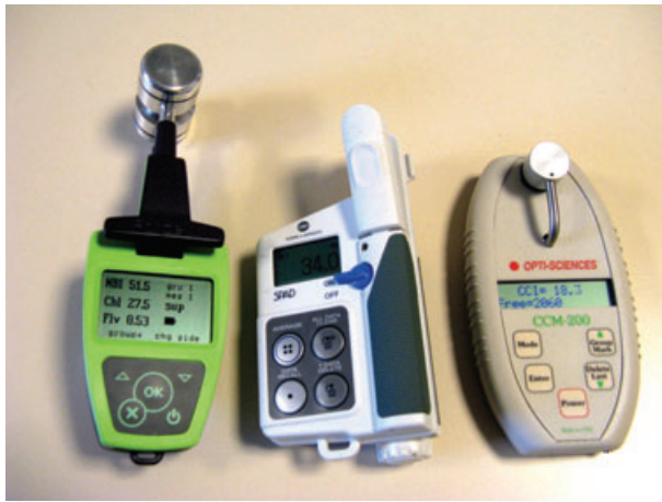
Fig. 1. Leaf-clip sensors used in this study. From left to right: Dualex 4 Scientific, SPAD-502 and CCM-200.
