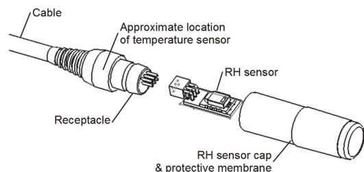
4. Push gently but firmly to install the new sensor (HUM-RHPCB-2) **in the same orientation.**
